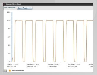
Performance analytics can be used to identify zone data points that indicate a failure to operate correctly – this example of a conference room occupancy sensor that never changes state during daily occupied periods warrants further investigation to determine the root cause of the failure
