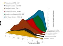
Maximum specific growth rate as a function of temperature for six different microalgae strains. Temperature tolerance and optimum temperature differ markedly among strains.
