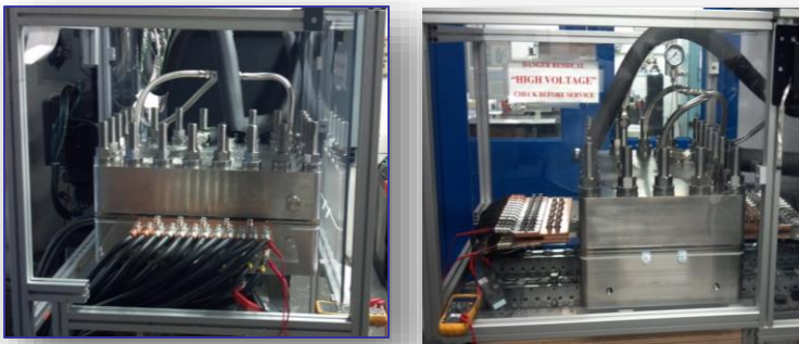
Short-stack testing of Giner's MW platform, 100 kW required for 6 cells, weight 2500 kg
