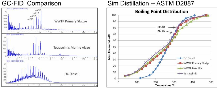
Sim Distillation -- ASTM D2887
