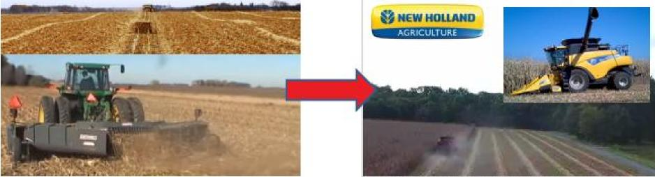
Separate shredding operation; ~ 2 ton/acre or more Shredding in new header; Optimized biomass removal rates; Avoids separate shredding operation
