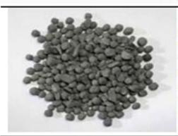
Direct Reduced Iron: DRI is typically produced in pellet form and can be loaded directly into an EAF, Blast Furnace, or Basic Oxygen Furnace. It contains a very high iron content (typically >90%). DRI exits the DRI module at a high temperature, and can be fed directly into furnaces as a means to reduce energy costs.
