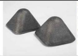
Merchant Pig Iron: MPI is produced in a blast furnace and cast into small "pigs" suitable for transportation. MPI has a higher iron content (around 96%) and less slag elements than DRI or HBI, and will typically sell at a premium. That said, MPI, HBI, and DRI are all substitutes for one another.
