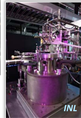
TAP reactor for extracting quantitative kinetic data
