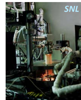
Stagnation flow reactor to evaluate kinetics of redox material at high-T
