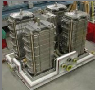
Four-Stack Module 1.4 megawatts
