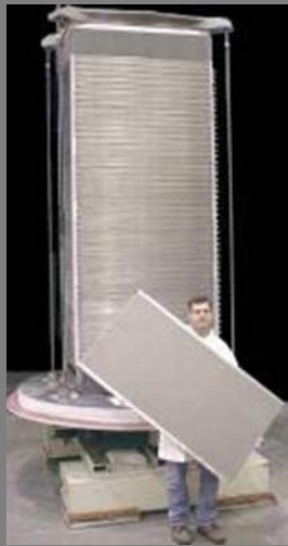
Individual fuel cell & 350 kW fuel cell stack
