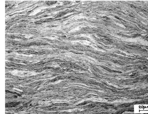
Cross section of compressed expanded graphite sheet
