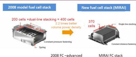
Maximum Power Volumetric power density Cell number of cells thickness of cell flow channel 90kW 1.4kW/L, 0.83kW/kg 400 cells, dual line stack 1.68mm straight channel MIRAI FC stack 114kW 3.1kW/L, 2.0kW/kg 370 cells, single line stack 1.34mm 3D fine-mesh flow field
