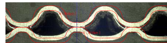
Stretch-formed bipolar plate dimensional conformance. Examples taken from full sized bipolar plate samples.
