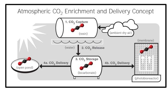
3. Uses bubble-less  $CO_2$  delivery: >90% into media, >70% into biomass
