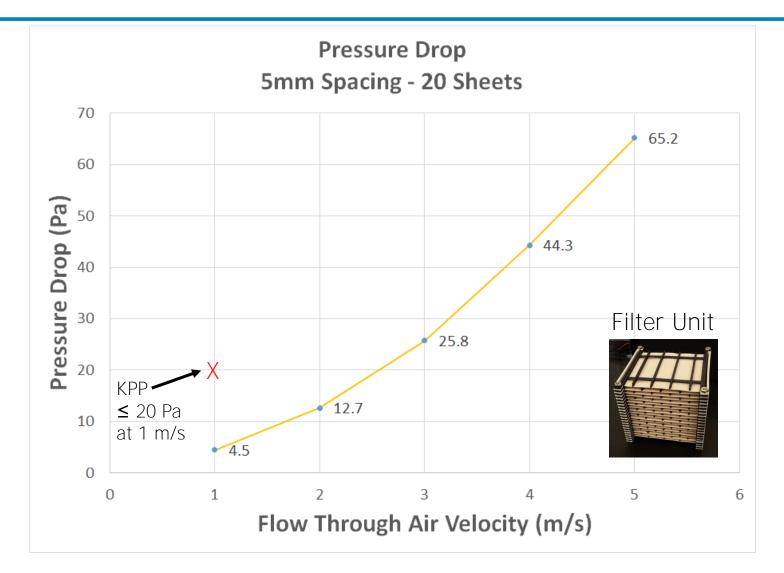
• Low pressure drop ensures sufficient air flow at low wind speed
