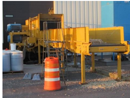
15 ton/hr 1st-Stage Grinder
