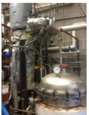
Bench Scale Extraction Reactor (Flow-Through) Dionex ASE350
