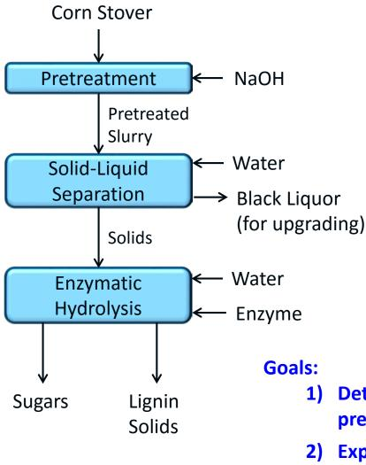
Pilot-scale alkaline pretreatment was researched as one method of obtaining soluble lignin for valorization (with Lignin Utilization project).
