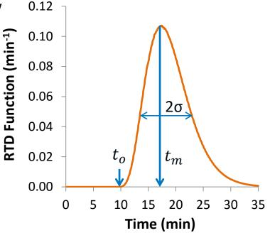
t<sub>o</sub>: Theoretical residence time (breakthrough time) based on screw speeds assuming no material slippage
