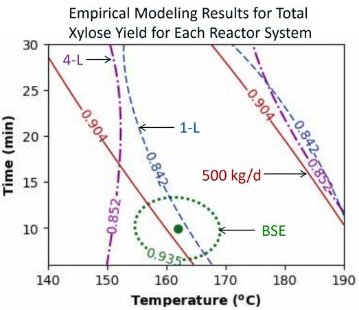
Plot shows the predicted maximum total xylose yield (96%) for the BSE reactor (green point) and yields at two standard deviations from the optimum for all reactor systems.
