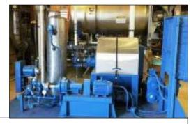
Acquired and reconditioned a used rotary drum filter; testing on enzymatic hydrolysates is under way.
