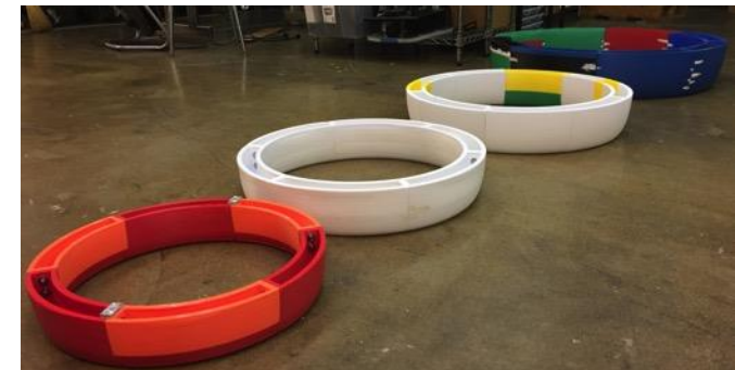
3D Printed Heave plates at 1:36 to 1:75 scales
