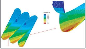
Optimized Composite Prototype for Archimedes Turbine Manufacture
