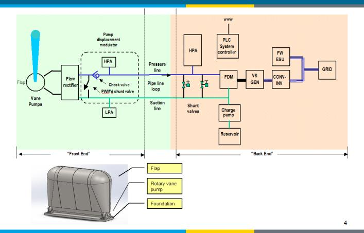
Optimal Control of a Surge-Mode WEC in Random Waves
