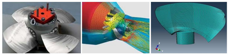
The Design and Development of a Composite Hydropower Turbine Runner
