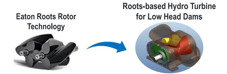
Cost-Optimized Modular Helical Rotor Turbine-Generator System for Small Hydro Power Plants
