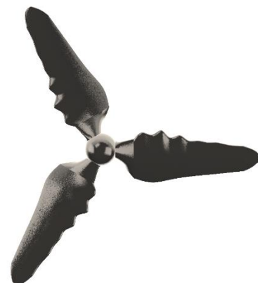
Figure 6. SolidWorks render of tubercle designed blades (Blade Design 3)
