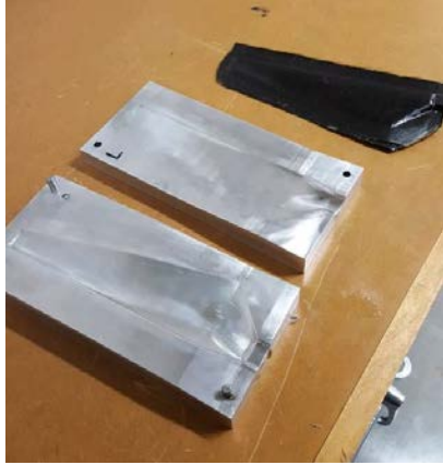
Figure 13. LEFT. CNC Machined Aluminum Turbine Blade Mold
