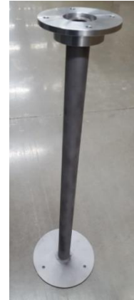
Figure 10. Tower assembly for prototype wind turbine
