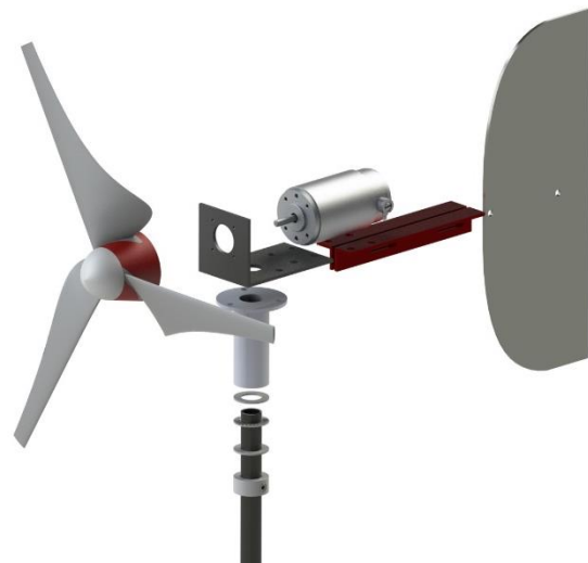
Figure 13: Upper Assembly Exploded View
