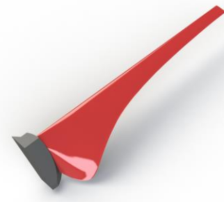
Figure 7: Rotor with S834 Airfoils and Optimized Chord and Twist Distributions
