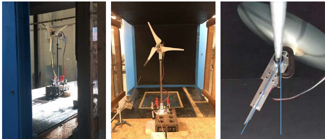
Figure 23: Wind Turbine in testing Tunnel
