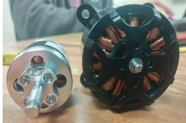
Figure 15: Comparison of motor size between last year (left) and this year (right)
