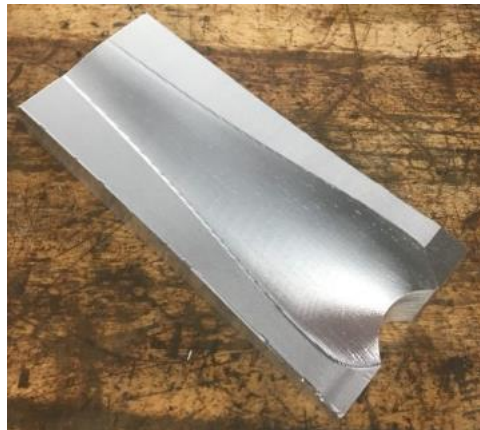
Figure 27: Aluminum Mold for Composite Layup Blades
