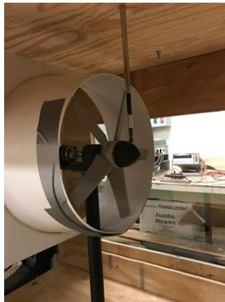
Figure 2. Test configuration of shroud prototype.
