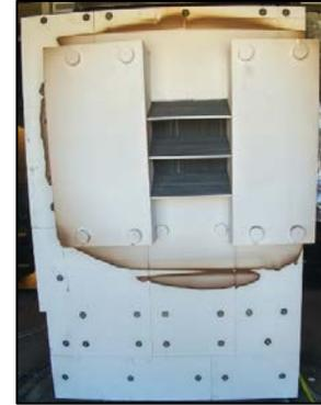
**Figure 45. Bladed receiver in place after on-sun testing.**
