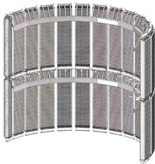
**Figure 34. Cutaway of an example surround-field receiver, comprising multiple absorber modules, each of which in turn comprises multiple unit cells aligned vertically and facing edge-out toward the incoming concentrated solar irradiance.**
