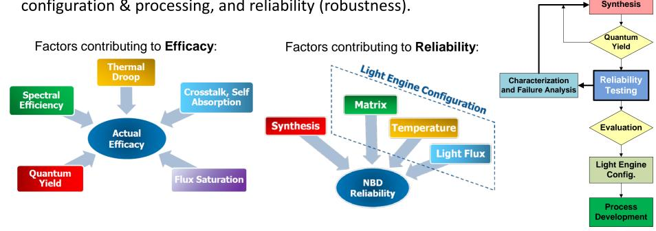
**Key Issues**: primary challenge is achieving high red NBD **reliability** in accelerated testing conditions (high light flux, T, & RH) while maintaining high **down-conversion efficiency** (*i.e.* turning blue photons into red photons).
