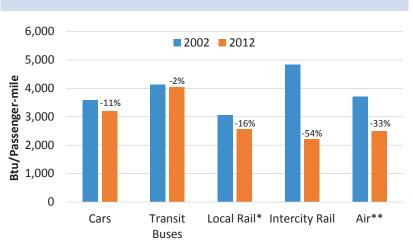
Figure 8.16 Energy per Passenger-mile by Mode in 2002 and 2012 with Percent Change from 2002 to 2012 Shown Above the 2012 Bars<sup>66</sup>
