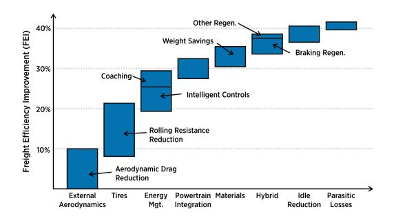
Figure 8.7 Vehicle-level Technology Contributions to Efficiency.<sup>28</sup> Freight efficiency represents decreased energy use per ton-mile.
