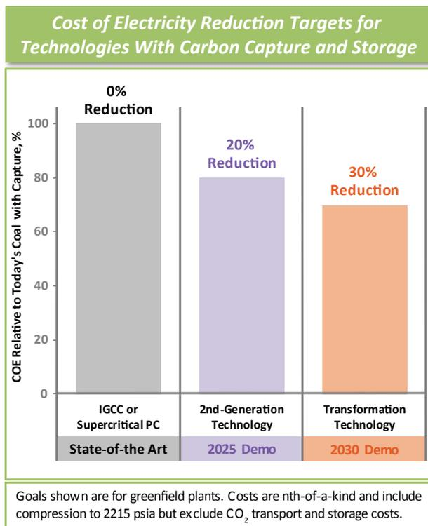
Second-generation CCS technology includes a suite of improvements in capture performance, plant efficiencies, and component cost, and expanded characterization of storage options. These technologies are expected to become commercially available in the mid-2020s. Analyses of coal power with CCS conducted by the National Energy Technology Laboratory (NETL) show a 20% decrease in costs of mature units compared to first-generation CCS technology.<sup>8</sup>
