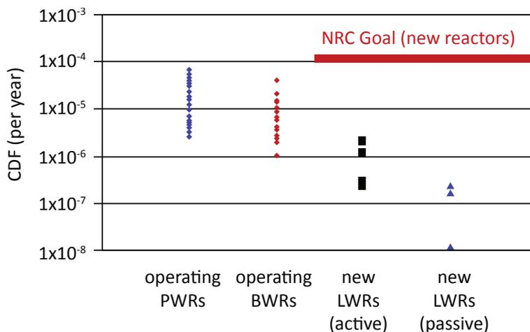
Values for new light water reactor designs with more passive safety features are one to three orders of magnitude lower.
