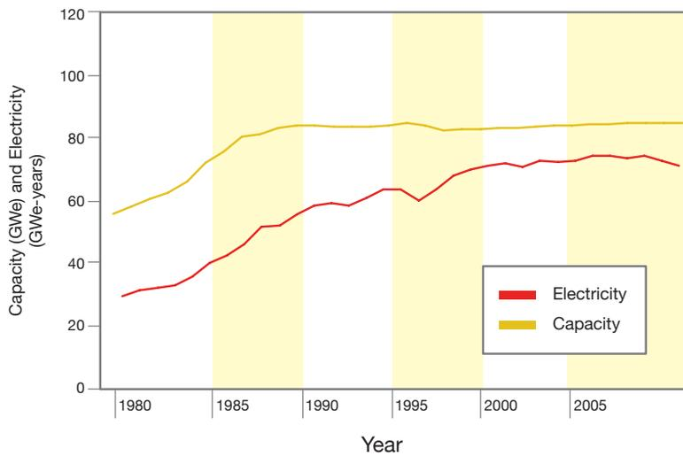
Even without additional new builds, the capacity and generation of nuclear power continued to increase due to power uprates and improved efficiencies.<sup>26</sup>
