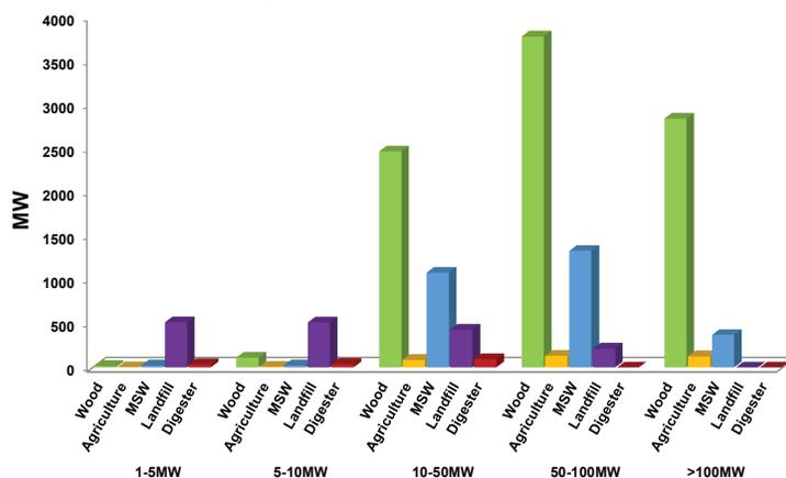
produced 64 million MWh of electricity. These units are typically fired with opportunity fuels such as sorted municipal solid waste (MSW), agriculture and wood residues, sewage sludge, and pulp and paper industry black liquor. The heat produced by the combustion of this biomass is converted to steam, which is typically used to drive simple Rankine power cycles. The typical rating for these plants ranges from 2–100 MWe as seen in Figure 4.11.<sup>56</sup>
