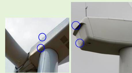
*Field Testing of Redesigned Deterrent Installed in Operating Wind Farm*
