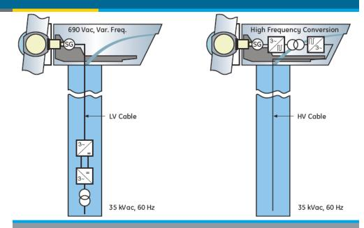
Left: a typical wind turbine contains power conversion elements down the post because of space requirements for the motor and gearing. Right: Innovative use of SiC-based HV power conversion allows all the necessary equipment to be co-located in motor housing saving on overall system costs. *Images courtesy of GE Global Research*
