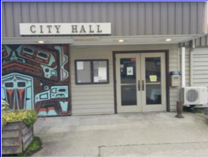
Wrangell City Hall in Southeast Alaska is heated by a heat pump.
