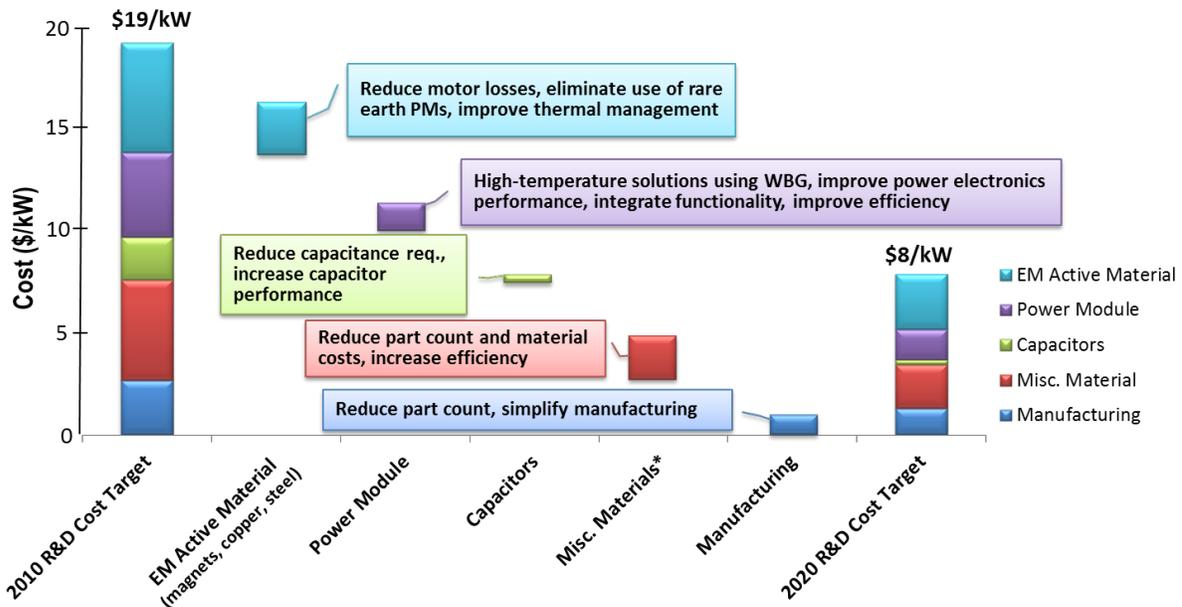
\* Inverter: cold plate, drive boards, thermal interface material, bus bar, current sensors, housing, control board, etc.
