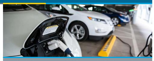
Workplace charging may be co-located with fleet EVSE or installed simultaneously to achieve cost savings. Here, an electric vehicle is plugged into a charging station in the NREL parking garage. *Photo by Dennis Schroeder, NREL 26669*
