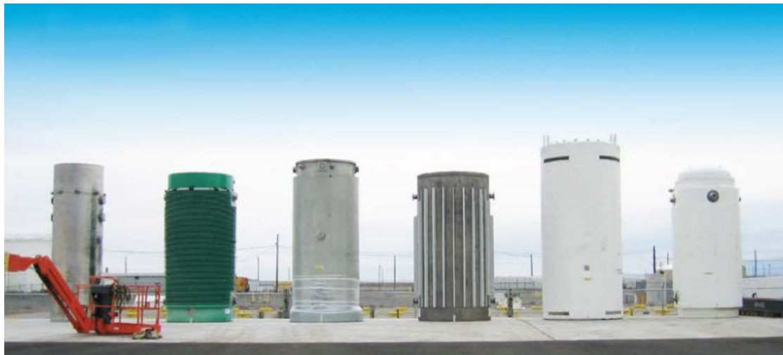
Figure 2-1. Dry Storage Casks at the Idaho National Laboratory INTEC Site. Left to right: NAC-I28, CASTOR V/21, REA 2023, MC-10, VSC-17, and TN 24P. (Photo courtesy of Idaho National Laboratory)
