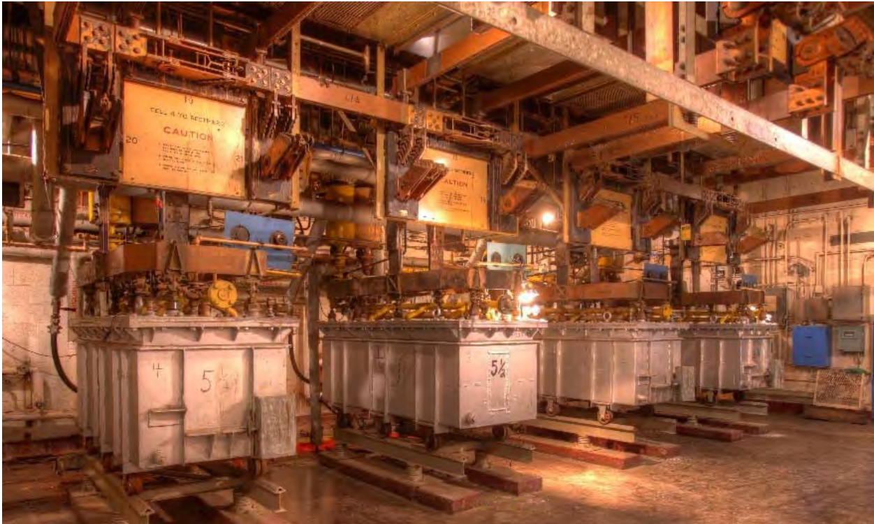
Figure 70. Fluorine Generation Units in the X-342A Feed, Vaporization, and Fluorine Generation Facility (1986)
