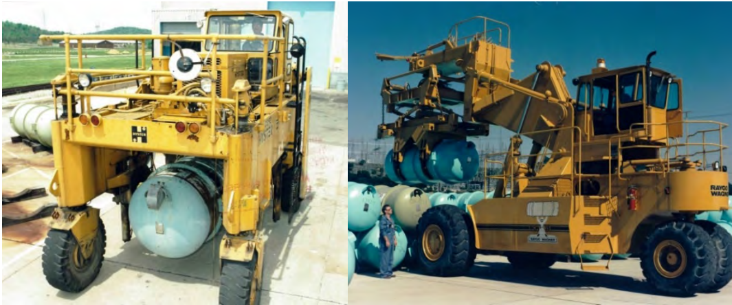
Figure 78. Cylinder Straddle Buggy (left) and Customized Crane Used for Transporting and Stacking UF 6 Cylinders (2009)
