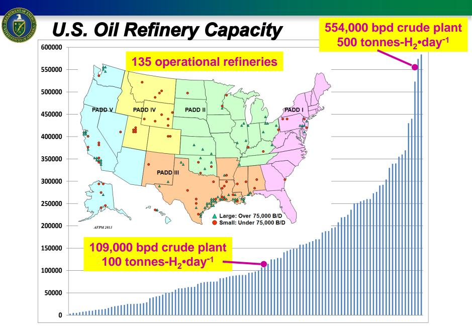
U.S. refinery operating capacity in barrels per stream day, as of January 2016
