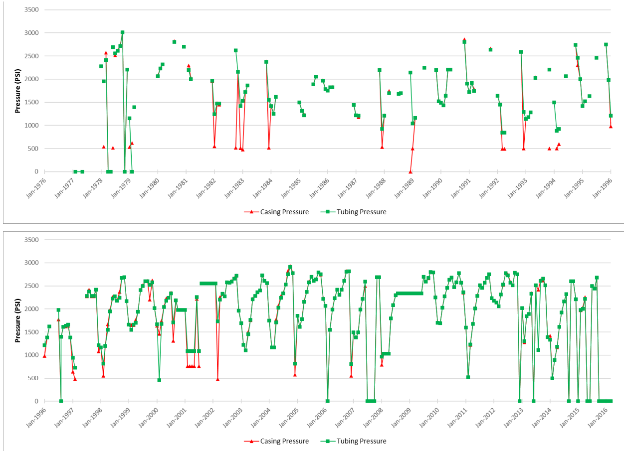
Figure 6: Casing and tubing production pressure history curves for Standard Sesnon 25.
