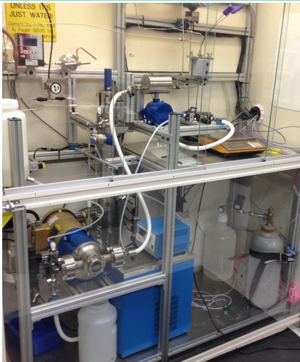
**Allows testing components (catalyst and membrane) and membrane electrode assembly collective properties for non-conventional electrolysis**
