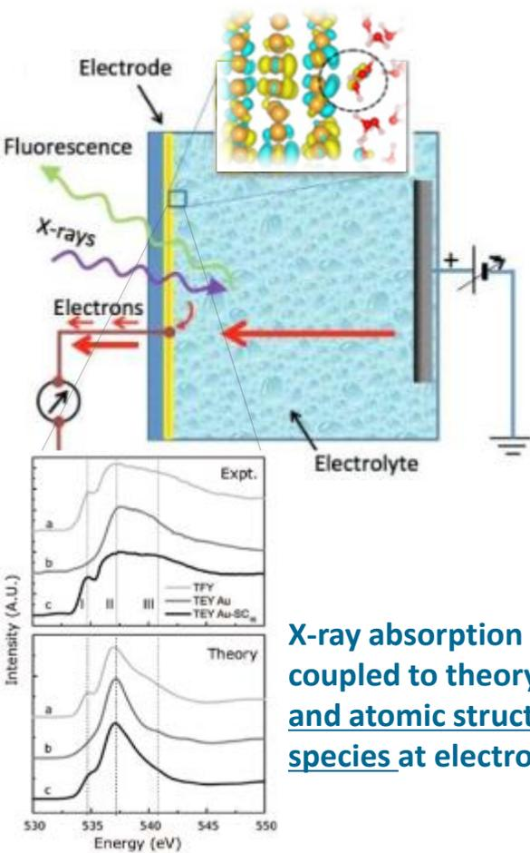
X-ray absorption spectroscopy, coupled to theory, reveals electronic and atomic structure of chemical species at electrode interface
