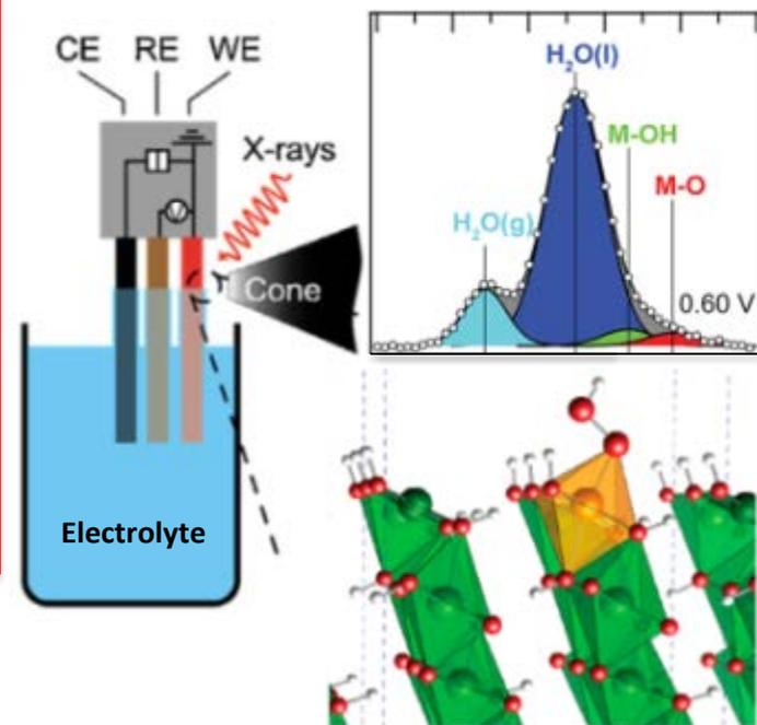
X-ray photoelectron spectroscopy and molecular simulations reveal atomic concentration, chemical speciation, and potential profile at electrode interface
