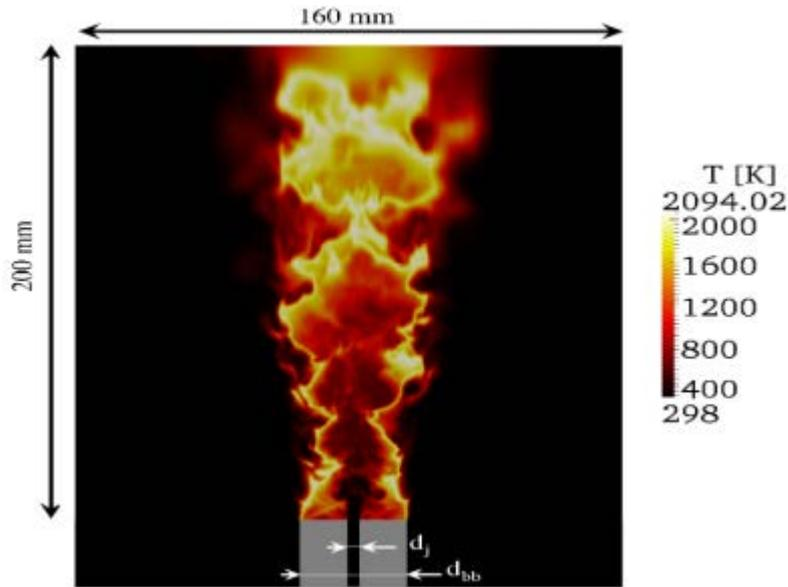
Large eddy simulations of turbulent combustion in a bluff body burner. UQTK was used for forward propagation of uncertainty in this system accounting for uncertainty in subgrid model parameters.
