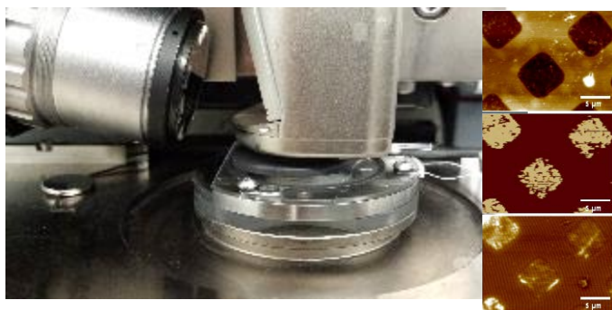
Left: setup for EC-AFM. Right: topography, contact current and electrochemical current of Au squares surrounded by a \text{Si}_3\text{N}_4 frame. 10 mM [\text{Ru}(\text{NH}_3)_6]^{3+} solution as electrolyte.
