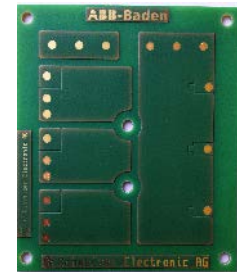
Next generation power electronics package
