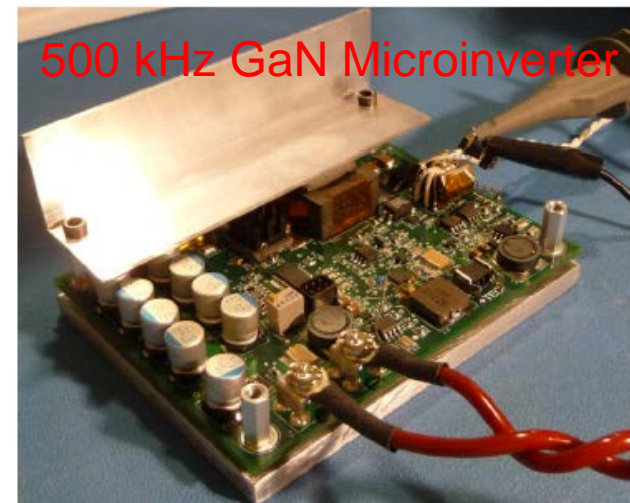
Fig 13: Prototype with thermal management employed during testing.
