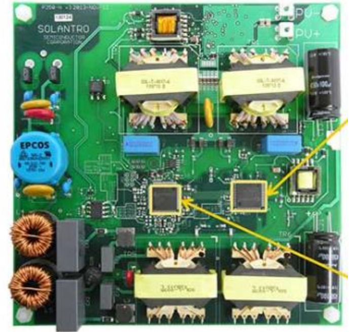
Solantro 350 W PV microinverter: Miniaturized control chips are great but passives are still huge.
