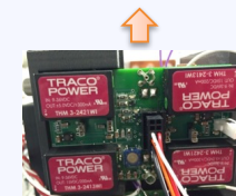
ORNL Gate Driver Board
