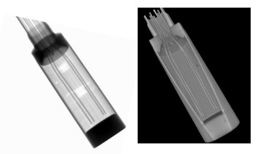
X-ray (left) and 3D CT (right) images of MPFD showing wire connections
