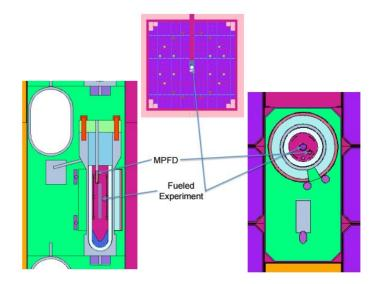
MCNP Transient MPFD model (left) and location in experiment (right)
