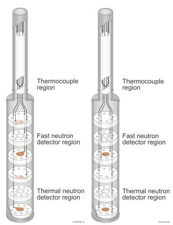
Parallel plate design (left) and parallel wire design (right)
