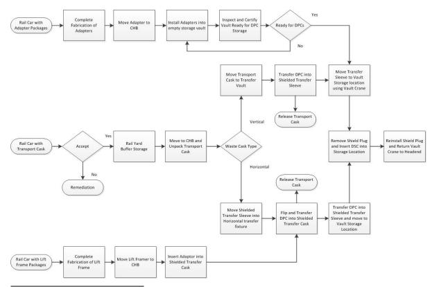
Canister Handling Material Handling Flow Diagram BGVa<sup>3</sup>
