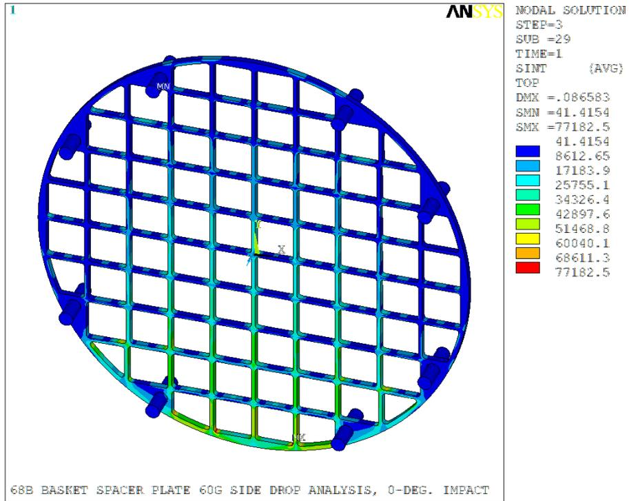
Figure 4-24. 68B Basket 60g 0° Side Drop S.I. Contour Plot
