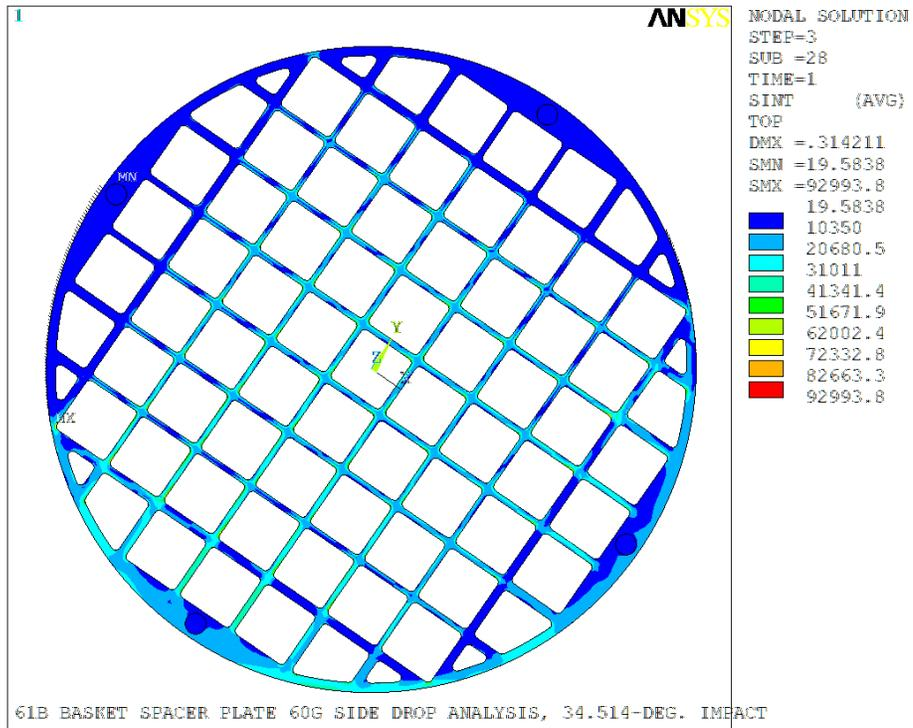
Figure 4-29. 61B Basket 60g 35° Side Drop S.I. Contour Plot
