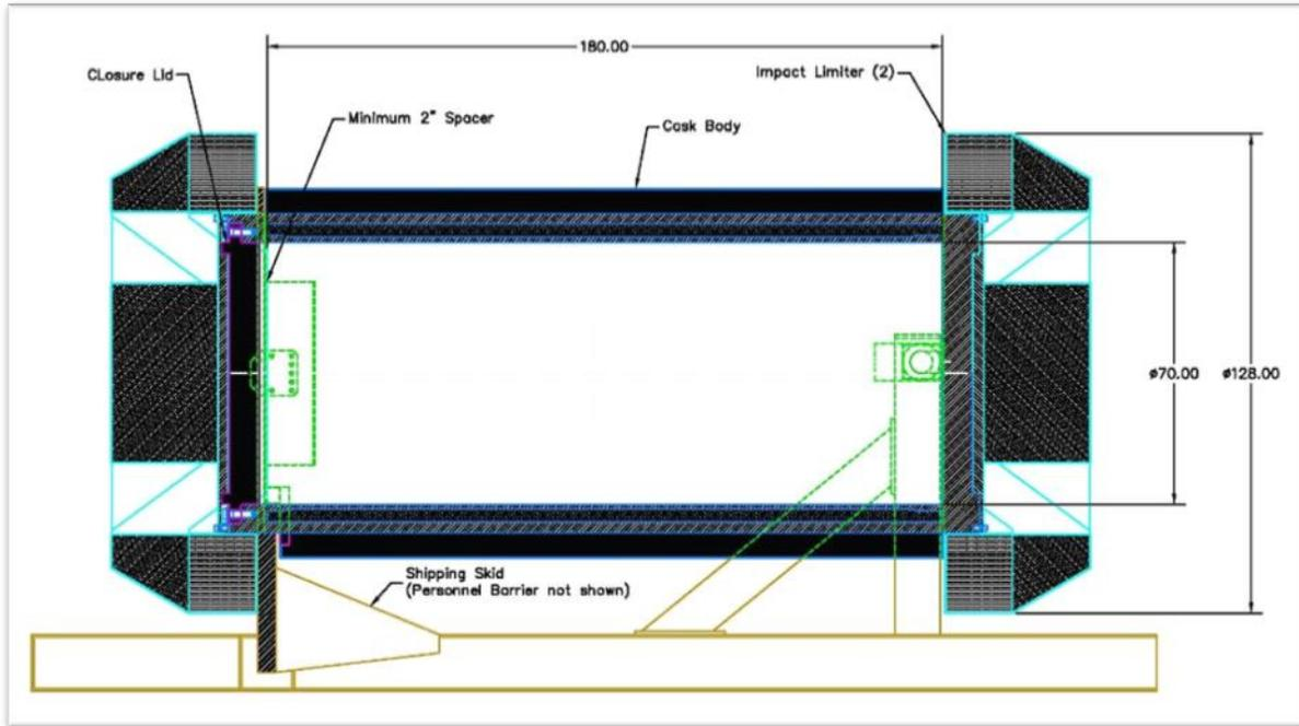
**Figure 4-1. Cross-Section View of the Regular Transportation Cask**
