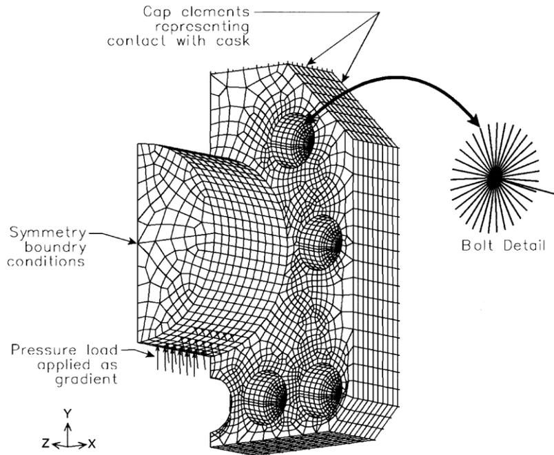
**Figure 4-12. Details of the ANSYS Model and Boundary Conditions**
