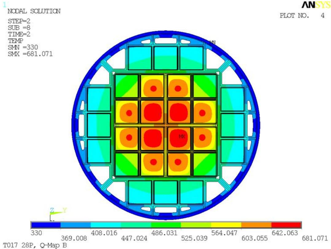
**Figure 4-42. Basket and Assembly Material Temperature Distribution – 28P Basket – Concentrated Payload**
