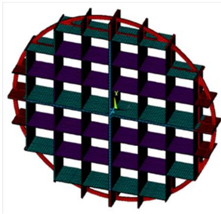
**Figure 4-15. 32P Basket Structural Model**
