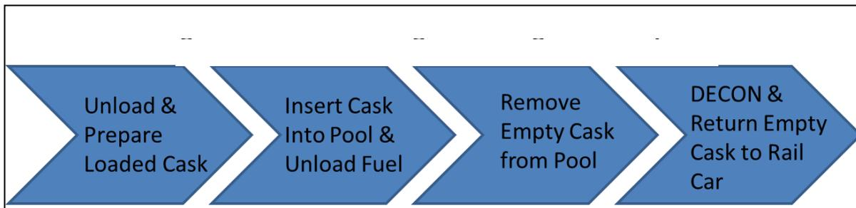
**Figure 10-2. Cask Unloading Process High-Level Steps**
