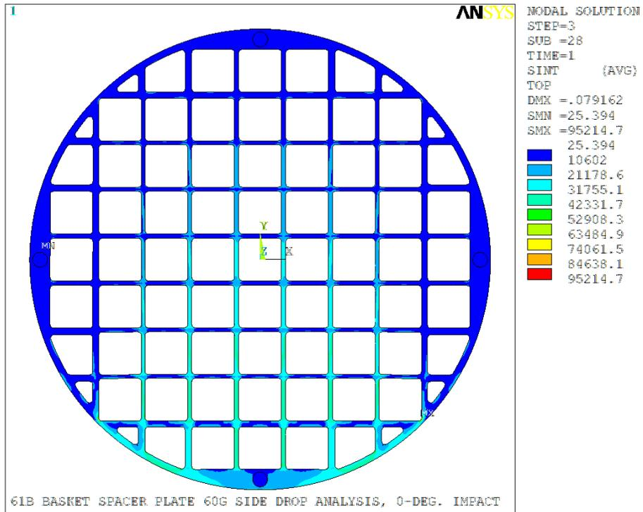
Figure 4-28. 61B Basket 60g 0° Side Drop S.I. Contour Plate
