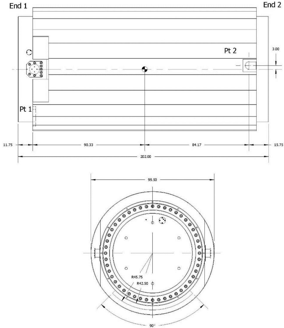
Figure 4-14. Side and End Views for the Transportation Cask
