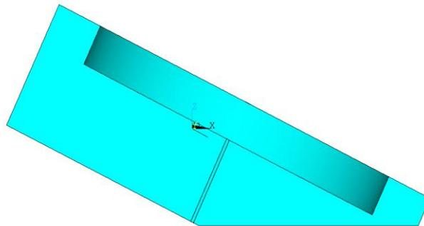
**Figure 4-11. Corner Drop – Approximated Deformed Shape**
