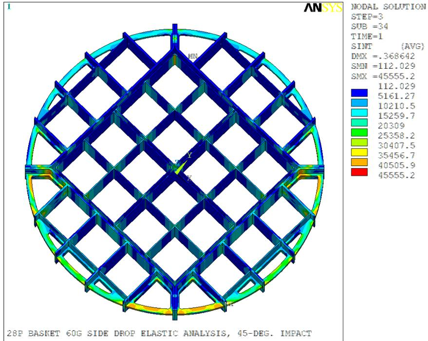
Figure 4-21. 28P Basket 60g 45° Side Drop S.I Contour Plot
