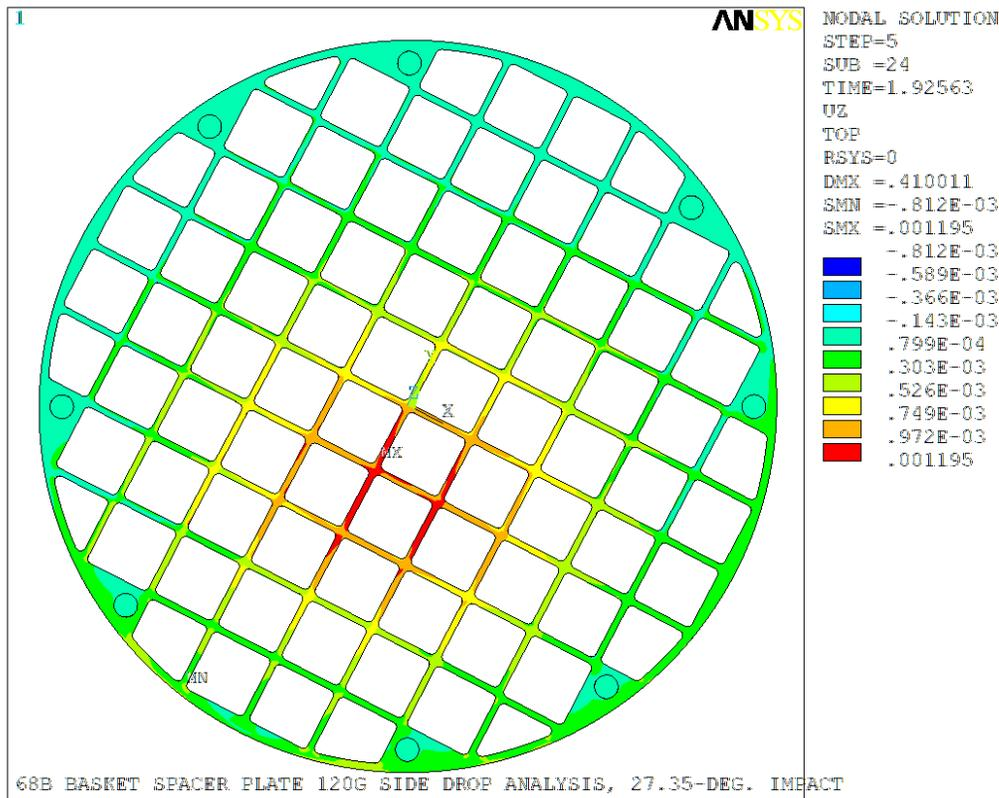
**Figure 4-26. 68B 27° Side Drop Deformations Preceding Plastic Instability Load**
