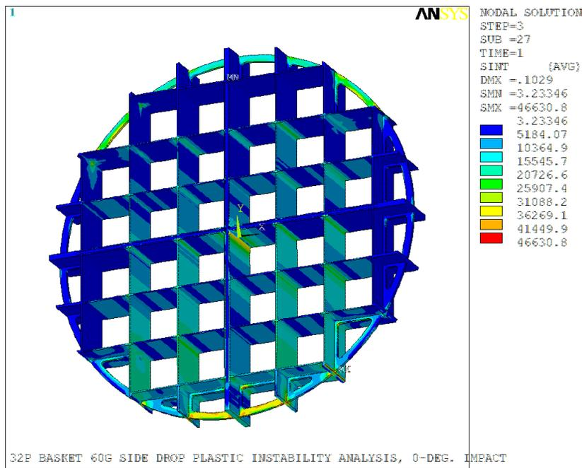
**Figure 4-16. 32P Basket 60g 0° Side Drop S.I. Contour Plot**
