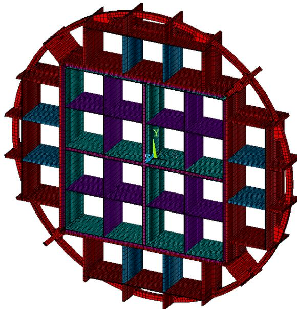
**Figure 4-19. 28P Basket Structural Model**
