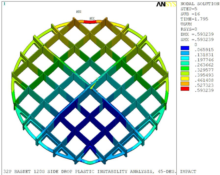
Note: Deformed Shape shown magnified 5×
