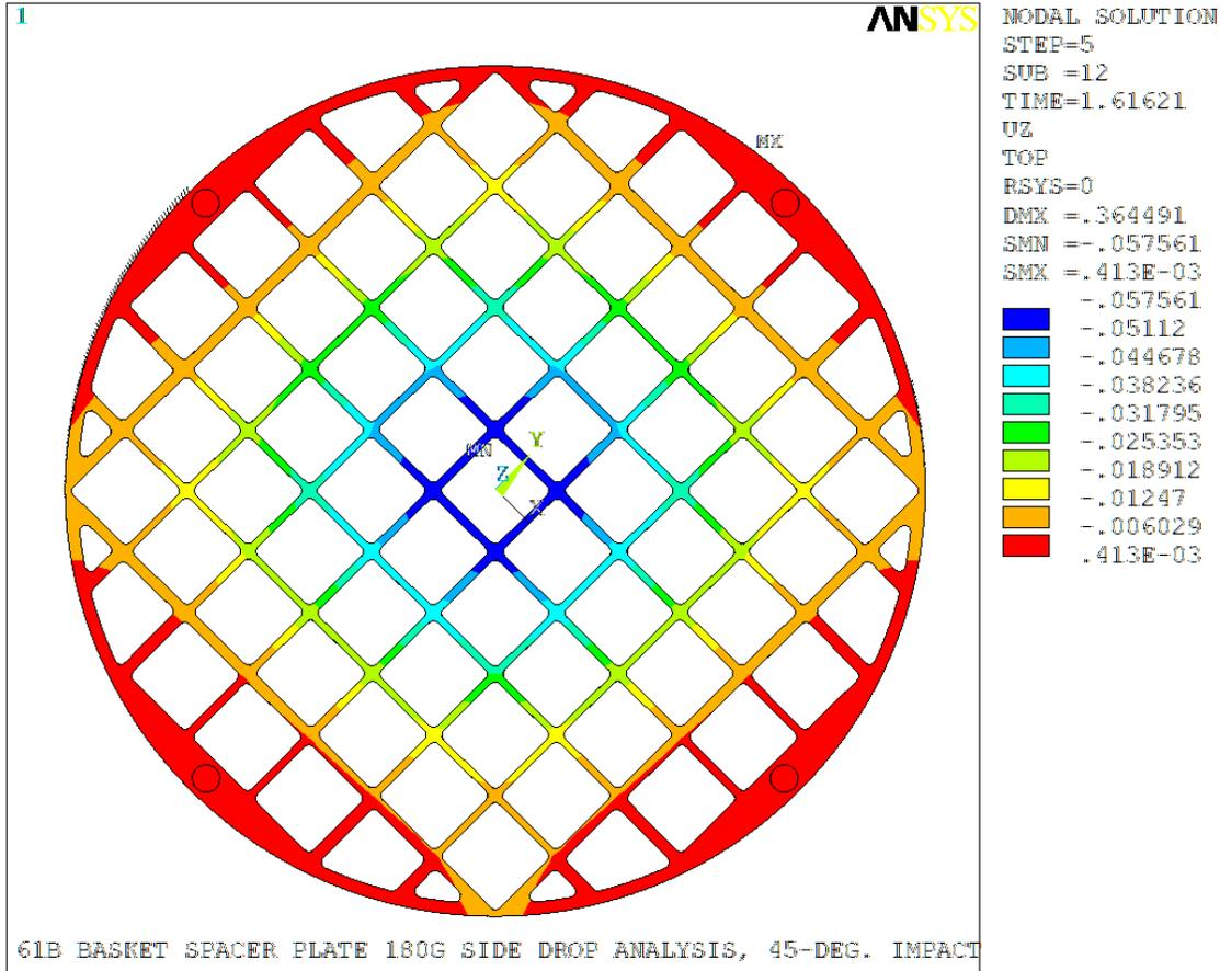
**Figure 4-30. 61B 45° Side Drop Deformations Preceding Plastic Instability Load**
