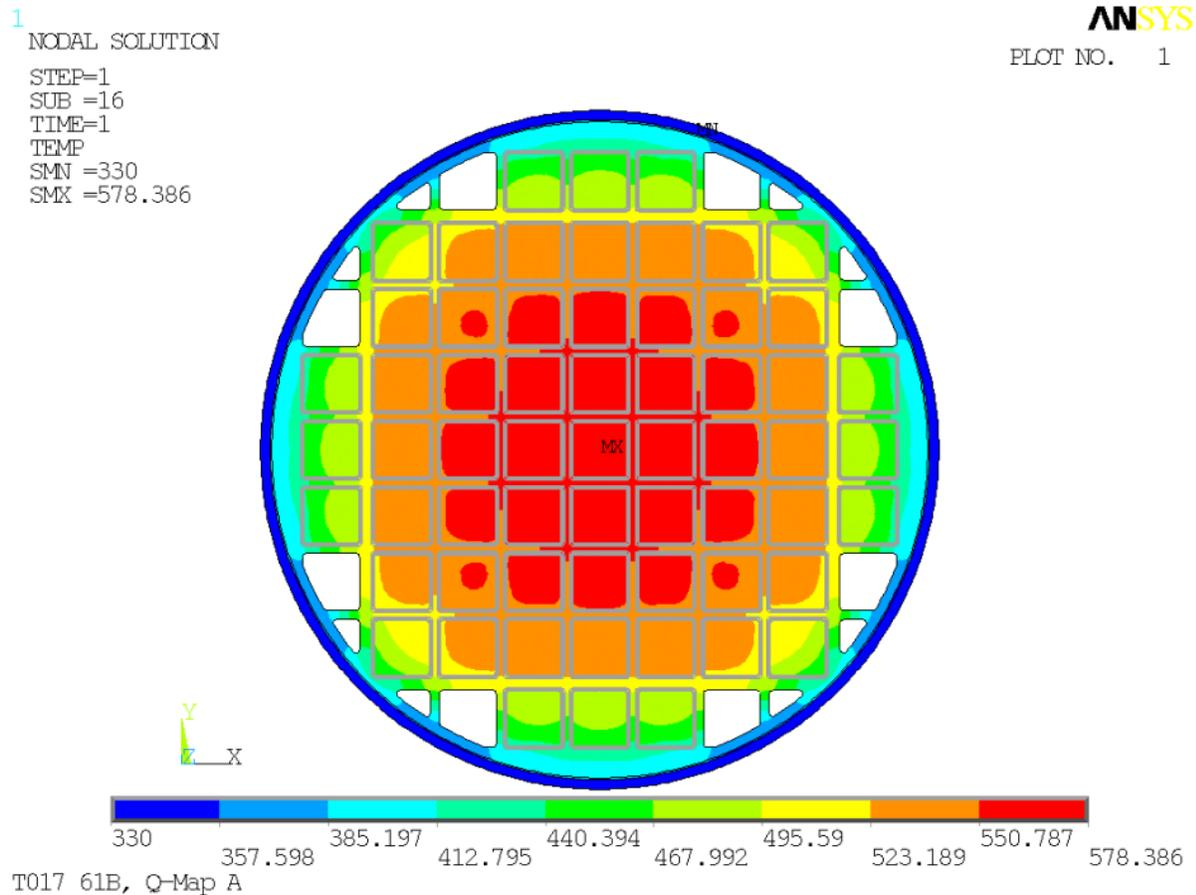
**Figure 4-45. Basket and Assembly Material Temperature Distribution – 61B Basket-Uniform Payload**
