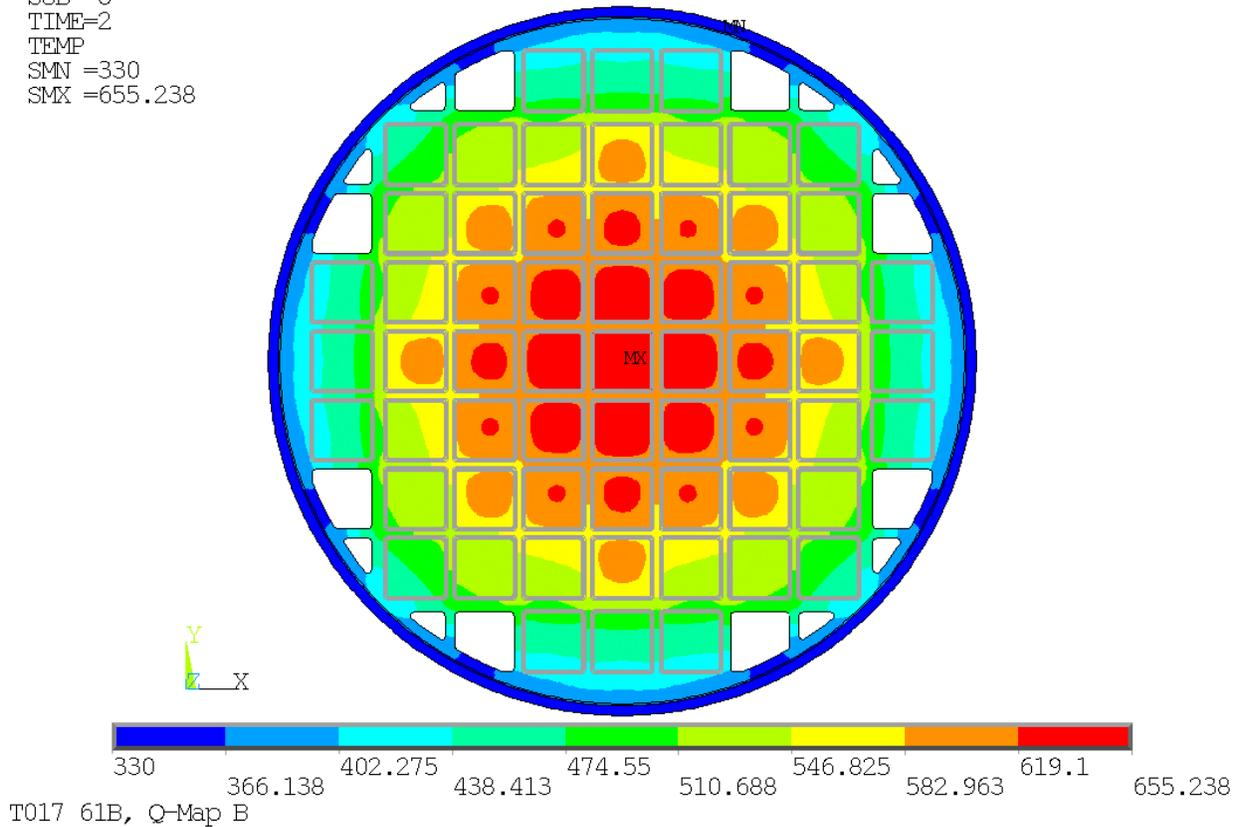
**Figure 4-46. Basket and Assembly Material Temperature Distribution - 61B Basket – Concentrated Payload**
