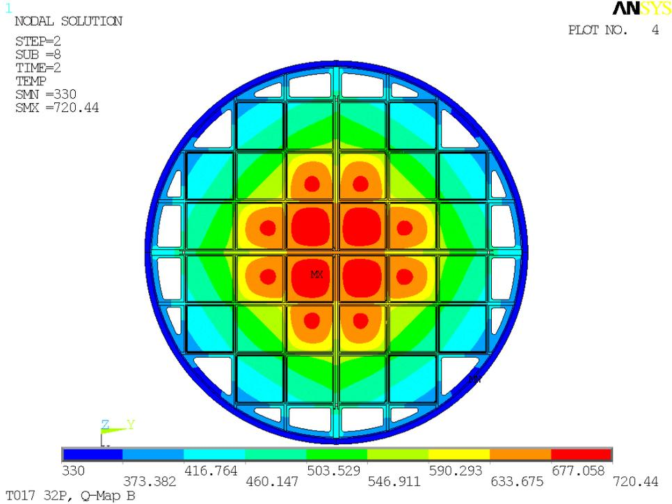
**Figure 4-40. Basket and Assembly Material Temperature Distribution – 32P Basket – Concentrated Payload**
