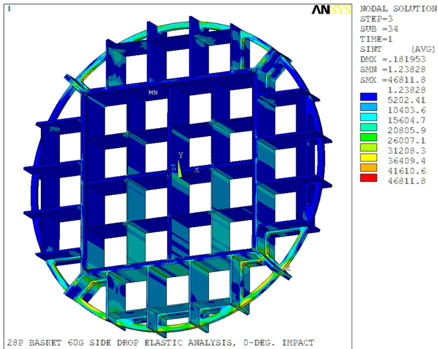
**Figure 4-20. 28P Basket 60g 0° Side Drop S.I. Contour Plot**
