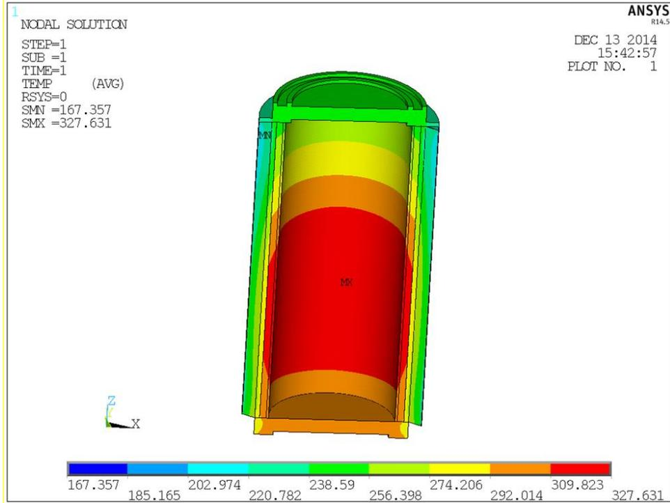
Figure 4-33. Thermal Gradients – Half-Symmetry Model for PWR Thermal Profile
