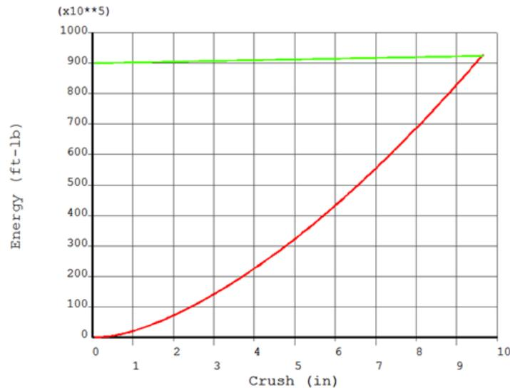
**Figure 4-10. Side Drop – Energy Dissipation by Crush Distance**
