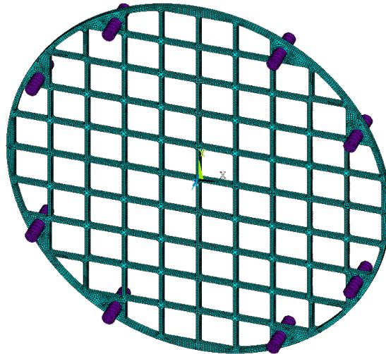
**Figure 4-23. 68B Spacer Plate Structural Model**
