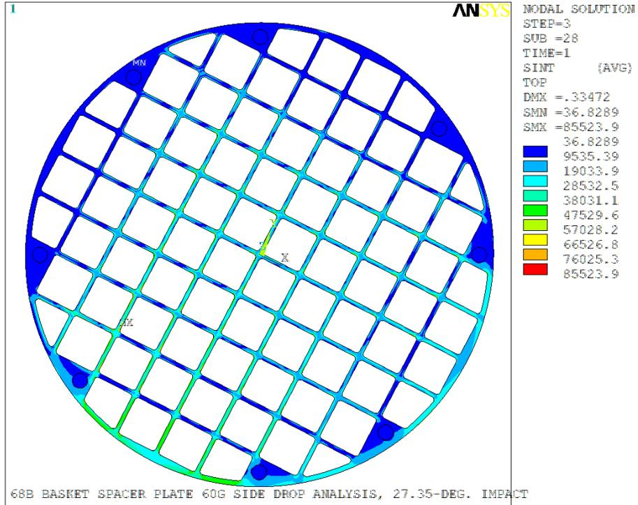
Figure 4-25. 68B Basket 60g 27° Side Drop S.I. Contour Plot
