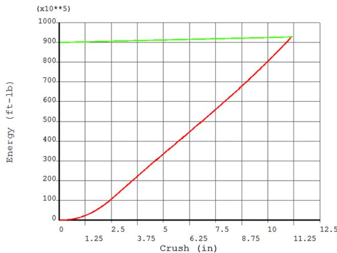
**Figure 4-9. End Drop – Energy Dissipation by Crush Distance**
