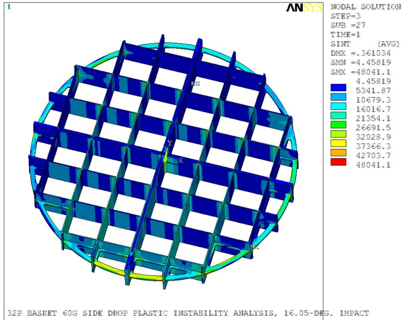
Figure 4-17. 32P Basket 60g 16° Side Drop S.I. Contour Plot
