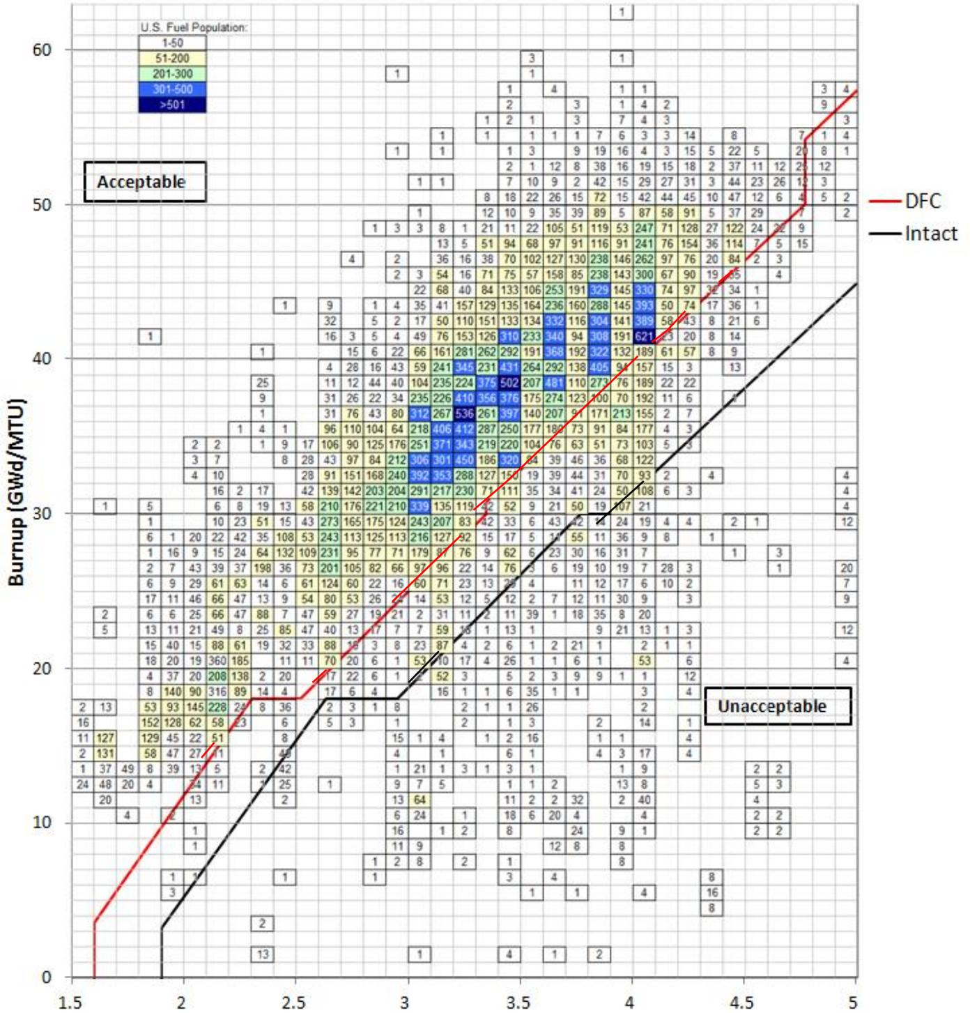
Figure 4-50. MAGNATRAN Intact Fuel and DFC Burnup Curves vs. US PWR Fuel Inventory
