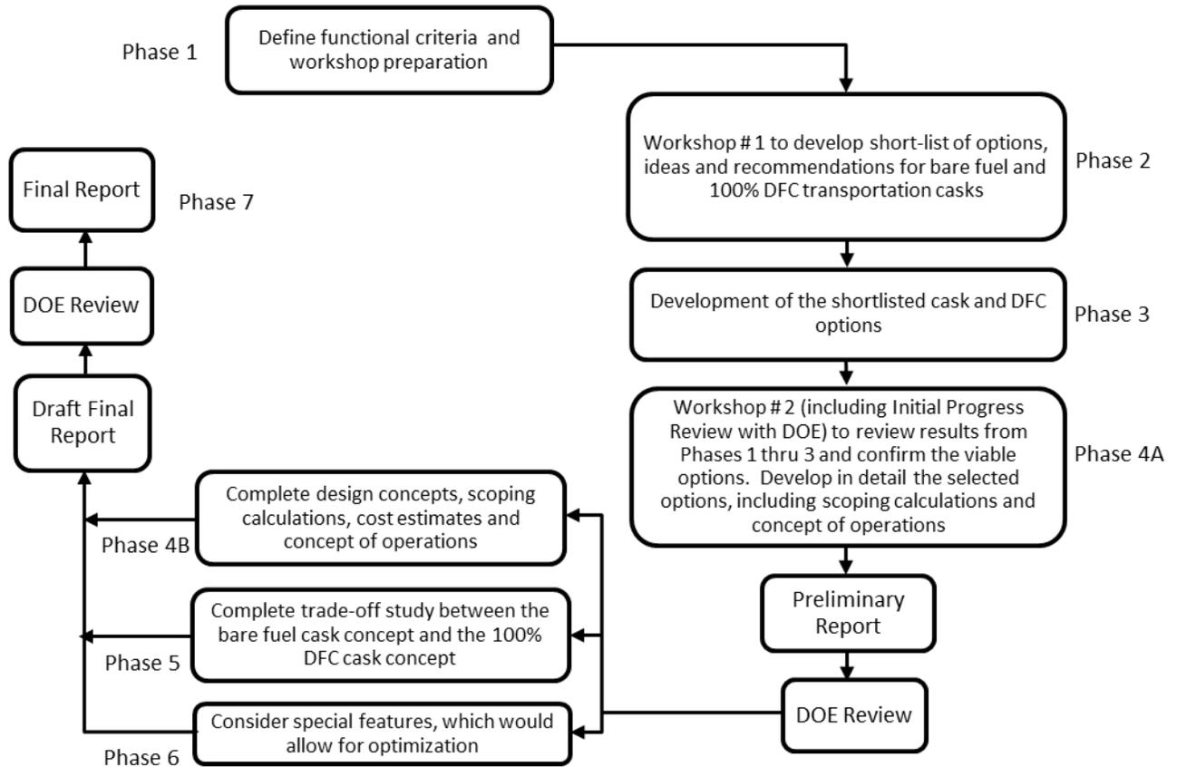
**Figure 3-1. Logic Diagram Showing Systems Engineering Approach.**
