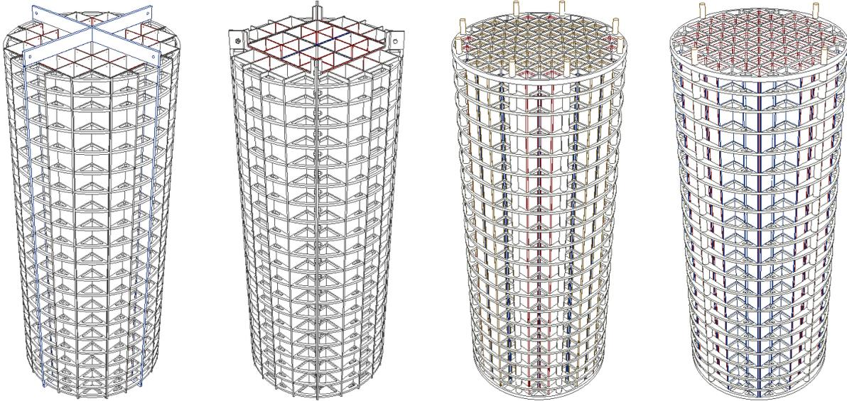
**Figure ES-4. Perspective Views (from left to right) for 32-PWR, 28-PWR, 68-BWR and 61-BWR Fuel Assembly Baskets**
