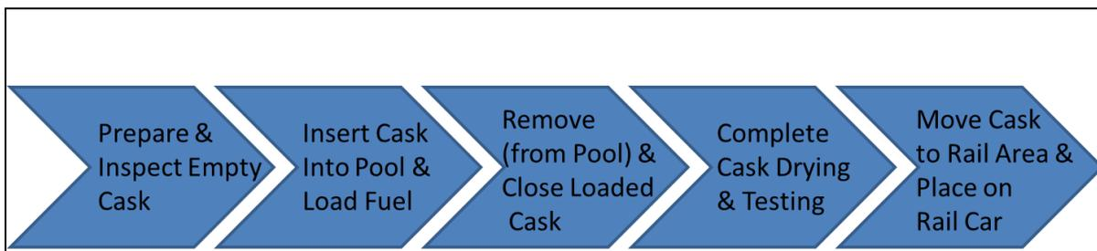
**Figure 10-1. Cask Loading Process High-Level Steps**
