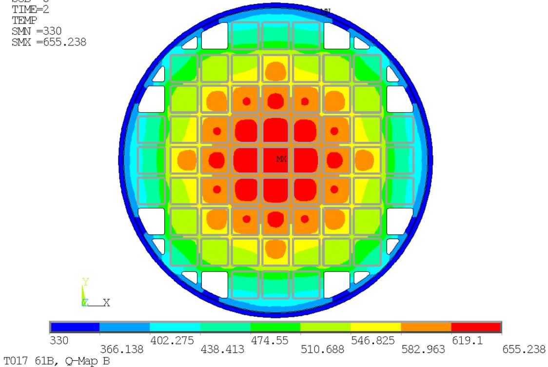
**Figure 4-44. Basket Structure Material Temperature Distribution – 68B Basket – Concentrated Payload**
