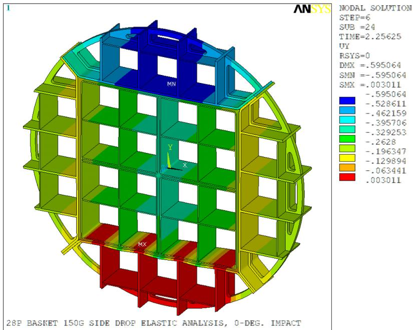
Figure 4-22. 28P 0° Side Drop Deformation Preceding Plastic Instability Load
