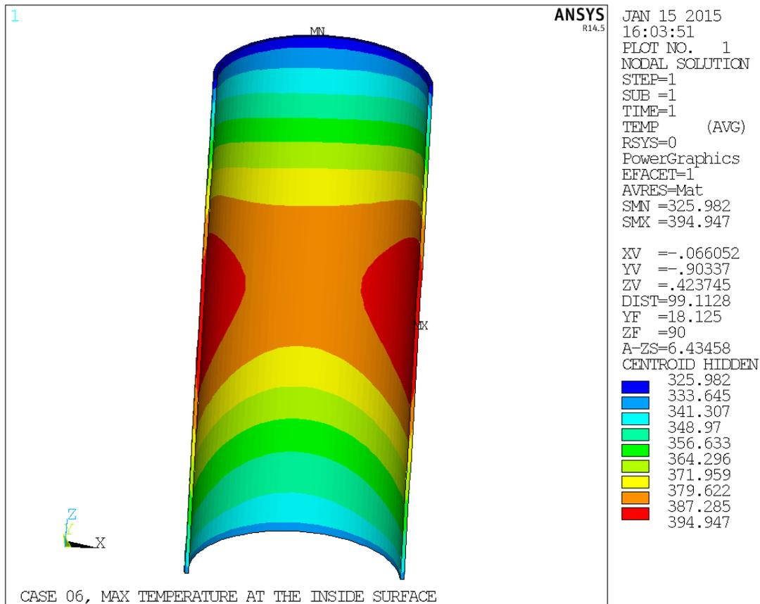
**Figure 4-37. Thermal Gradients – Half-Symmetry Model for BWR Thermal Profile**
