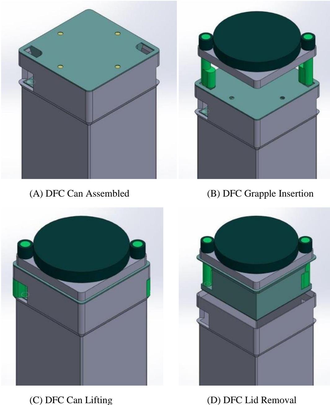
**Figure 4-8. Damaged Fuel Can Assembly for PWR Fuel**
