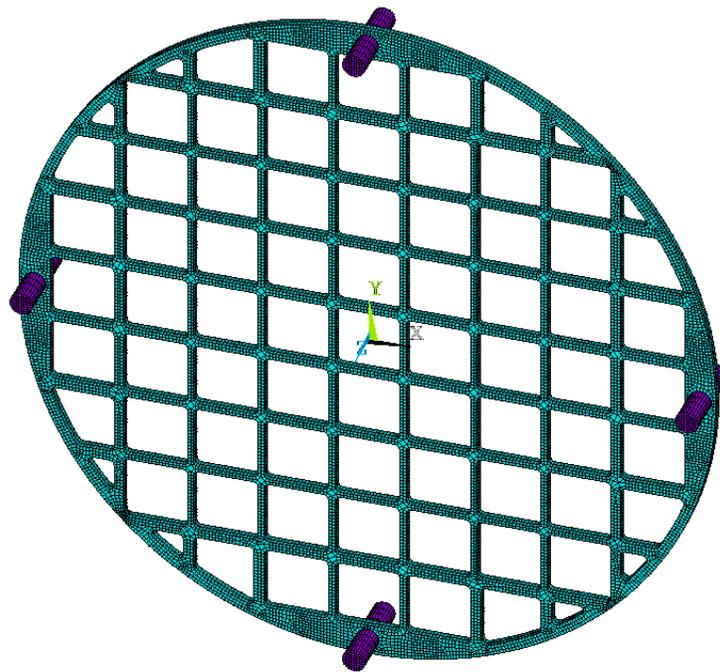
**Figure 4-27. 61B Spacer Plate Structural Model**
