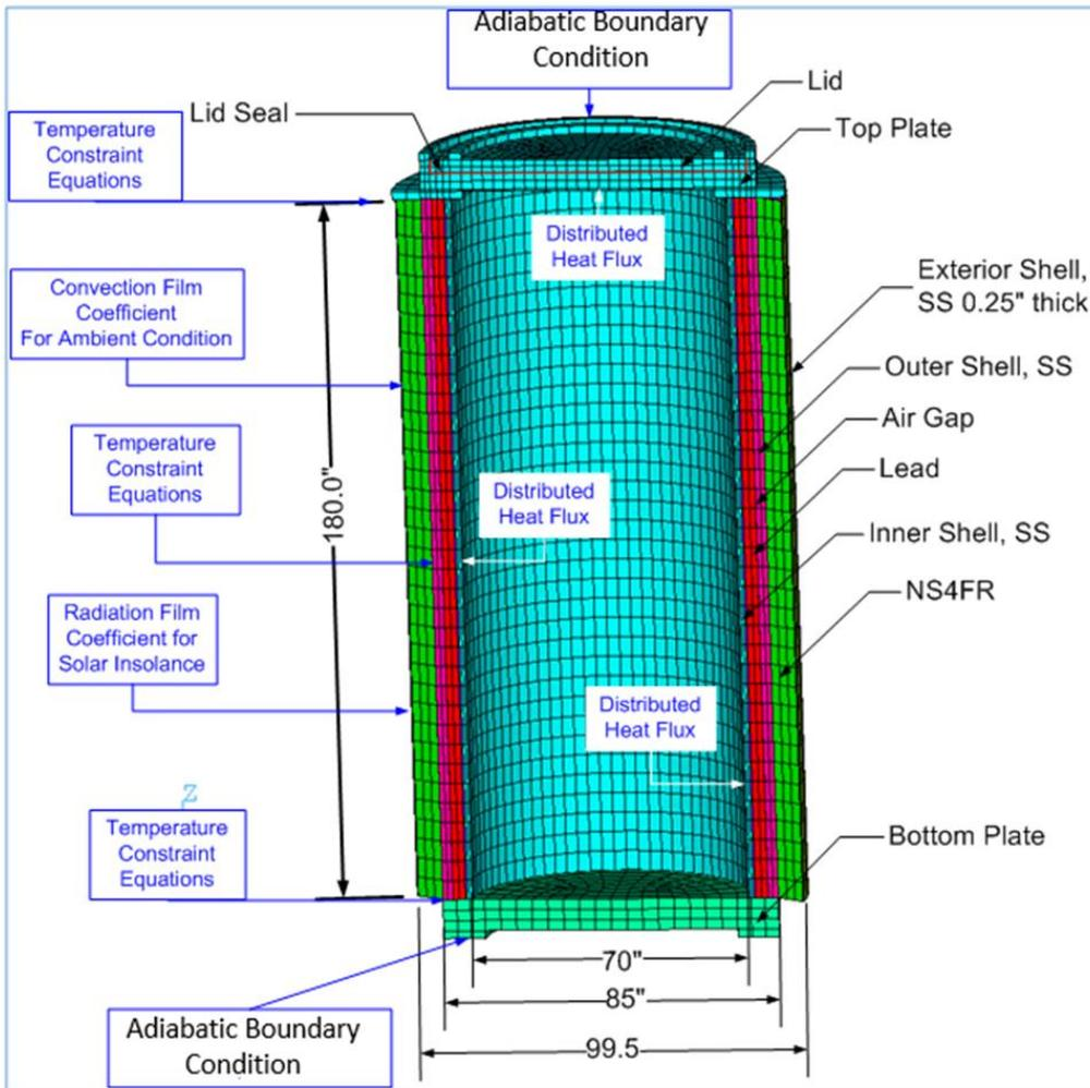
Figure 4-31. Thermal Boundary Conditions – Side View
