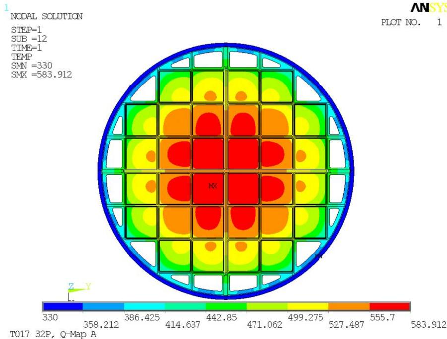
**Figure 4-39. Basket and Assembly Material Temperature Distribution – 32P Basket – Uniform Payload**
