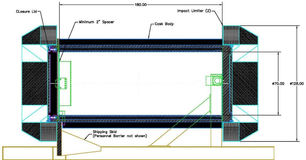
**Figure ES-3. Cross-Section View of the Transportation Cask**
