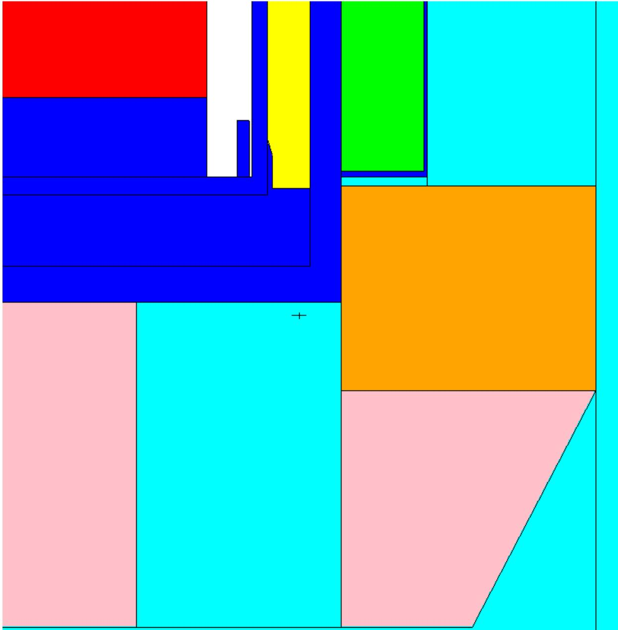
**Figure 4-49. Basket Bottom Corner Shield Ring Illustration**
