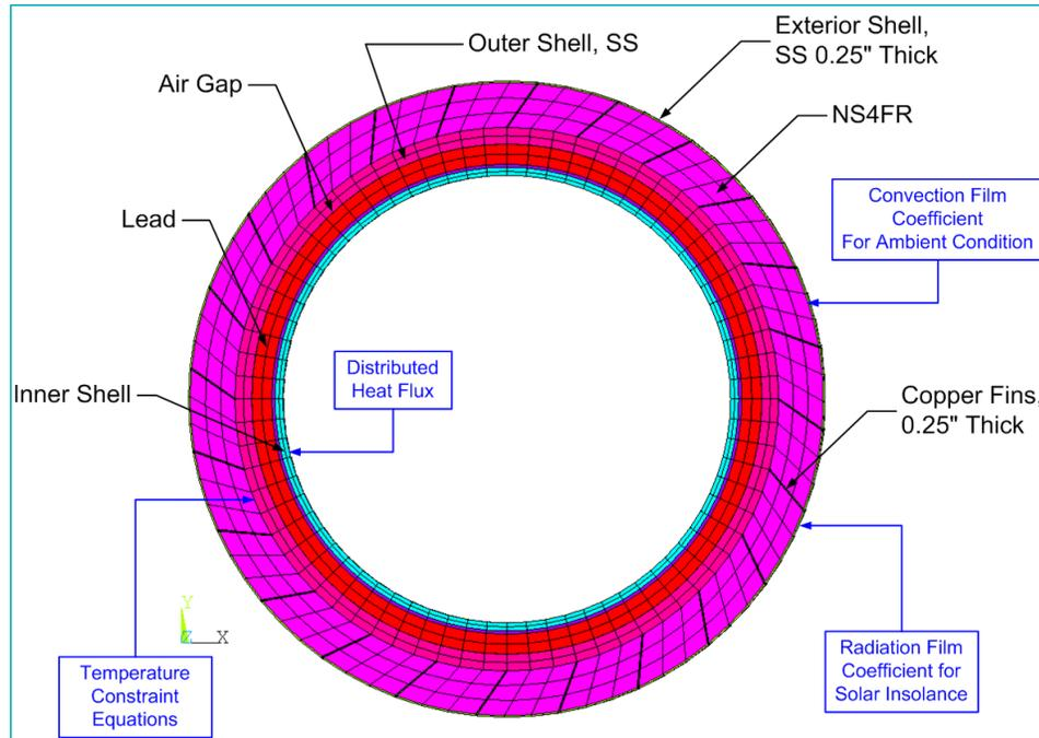
**Figure 4-32. Thermal Boundary Conditions – End View**
