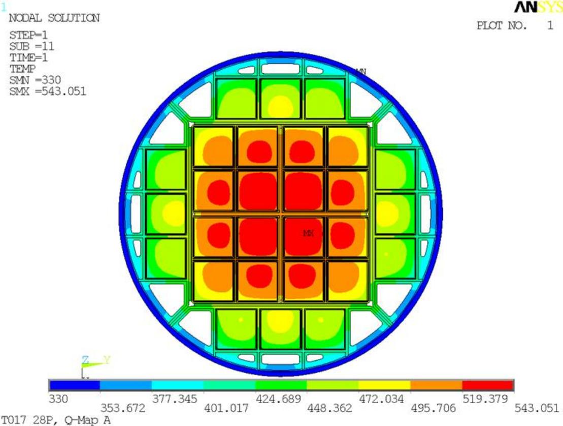
Figure 4-41. Basket and Assembly Material Temperature Distribution – 28P Basket – Uniform Payload
