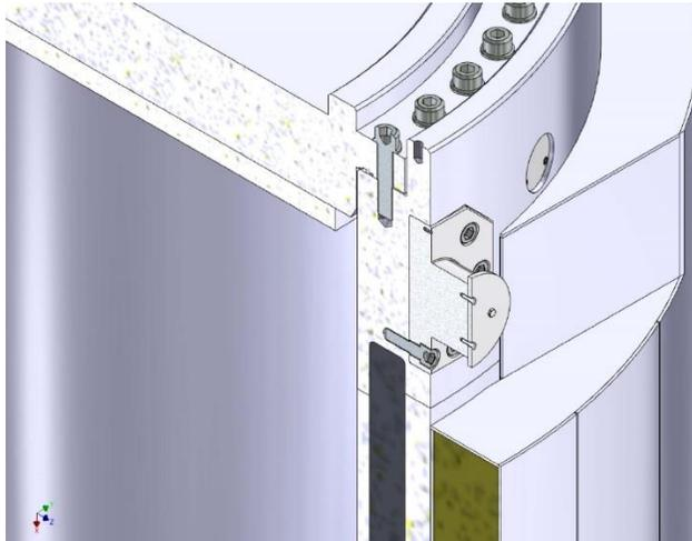
**Figure 4-2. Section View Showing Attachment of the Closure Lid to the Cask Body**
