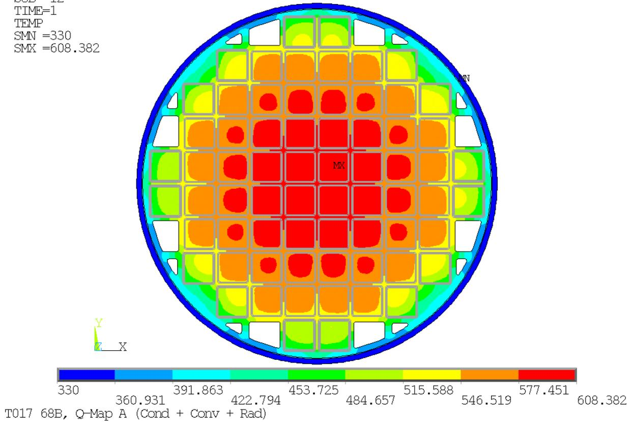
**Figure 4-43. Basket and Assembly Material Temperature Distribution – 68B Basket – Uniform Payload**
