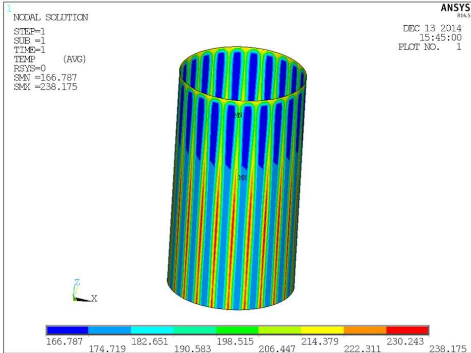
Figure 4-36. Evaluation of Junction of Thermal Fins and Neutron Shield Shell
