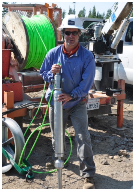
Figure J.12. Borehole seismometer, cable, and winch trailer used to install the NEGSD MSA.
