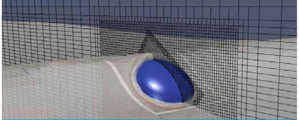
Computational fluid dynamics simulation of a WEC in focused waves.
