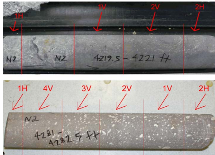
Figure A.30. Core samples from Well GEO N-2 from 4219.5 to 4221 ft MD (top), and from 4219.5 to 4221 ft MD (bottom) showing the location of 1 in. in diameter by 2 in. long sample plugs.
