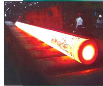
Hot extrusion of an Inconel® Alloy 740 (ASME Code Case 2702) pipe at Wyman-Gordon (PCC Energy), Houston, Texas. The 10,000-plus-pound ingot was cast by Special Metals Corporation, Huntington, West Virginia. Inconel® Alloy 740 is the prime candidate alloy for advanced ultrasupercritical steam boilers. (Photo courtesy of Wyman-Gordon)
